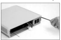
3. Slide the top of the system box to the rear and lift the top off.
