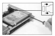
Disconnect the 4-wire connector from the backplane.
