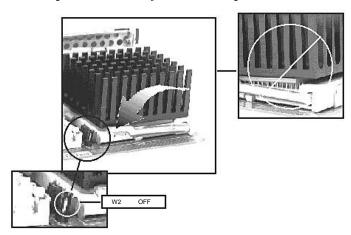
Set the W2, W4, W5, and W7 jumpers based on the Intel processor installed. See the System Board Jumpers section (page 103) for settings.
