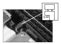
4. Disconnect the ribbon cable from the hard disk drive.
