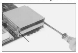
3. **Alpha-based models:** Disconnect the ribbon cable from the rear of the hard disk drive.
