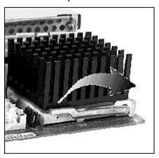
3. Lift the Intel processor straight up and out of its socket.
