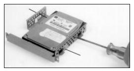
6. Lift the hard disk drive out of its frame.
