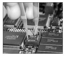
Save the Ethernet address ROM to install on the replacement system board.
