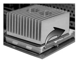
3. Lift the Alpha processor straight up and out of its socket.
