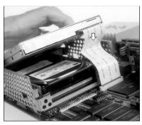
4. Remove the three screws holding the floppy disk drive in its frame, then slide the drive out of the frame.
