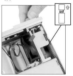
8. Use a screwdriver to release the clips holding the front bezel in place, then push the bezel forward about 0.5 inches.
