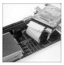
3. Lift the tabs of the floppy disk drive connector on the system board. Then disconnect the ribbon cable.
