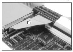
Remove the screw holding the backplane, then disconnect the backplane from its connector.
