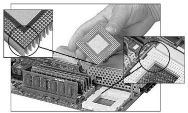
2. Lower the Alpha processor straight down into its slot, then lower the slot's handle and lock in place.
