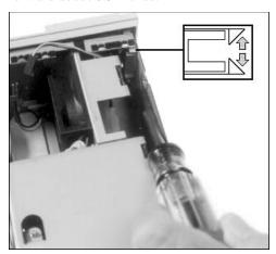
Disconnect the in-line speaker connector from the power supply.
