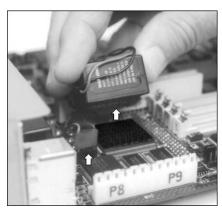
Intel-based models: The battery is on the underside of the system board. Lift the battery out of its seat.
