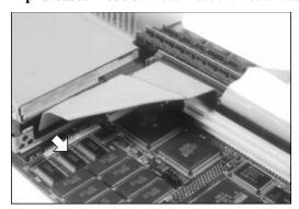
Intel-based models: Disconnect the ribbon cable from the rear of the hard disk drive and from the system board.
