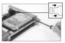
Disconnect the drive's 4-wire power connector and ribbon cable from the system board. Then disconnect the ribbon cable from the hard disk drive and lift the drive out.
