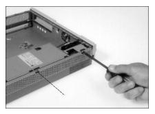
Disconnect the in-line connector on the cable for the power switch LED by lifting the connector's tab and pulling the two cable sections apart.
