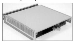
4. Remove the two screws holding the power supply to the system box frame.
