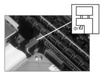
c. Lift the hard disk drive over the rear panel, out of the way.
