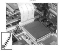
5. If the system has a SCSI-2 connector, remove the two screws holding the SCSI-2 connector on the rear panel. For model VX40, disconnect the other end of the ribbon cable, then remove the cable (part number 17-04124-01 shown) and connector. Models VX41 and VX42 have an integrated cable.
