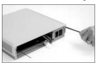
3. Slide the top of the system box to the rear and lift the top off.
