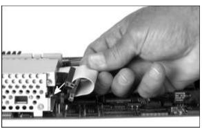
4. Slide the hard disk drive out of the card cage.
