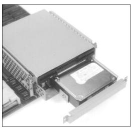
5. Remove the three screws holding the hard disk drive in its frame.
