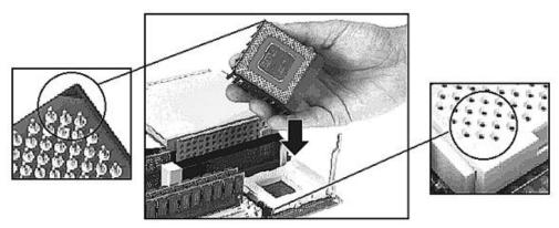
2. Lower the Intel processor straight down into its slot, then lower the slot's handle and lock in place.
