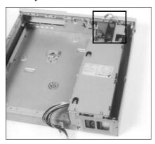
7. Push the rear end of the power switch shaft forward to disconnect it from the power supply shaft.
