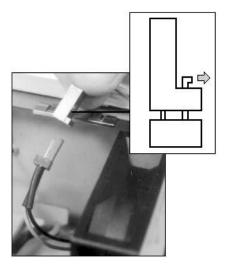
Slide the power supply about 0.25 inches toward the center of the system box and carefully route the LED wires behind the fan housing.
