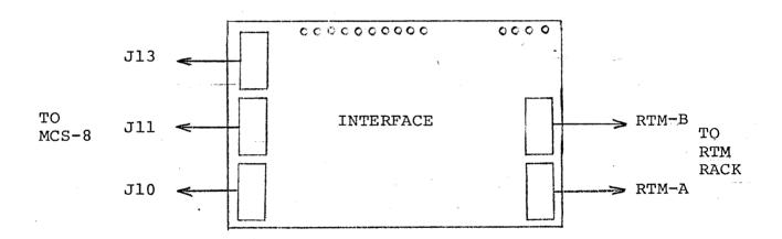
Connectors to the MCS-8 are 16 pin dip cables. Those to the RTMs have 16 pin dip on one end and RTM cards on the other end. Make sure the dip plugs are oriented properly.
