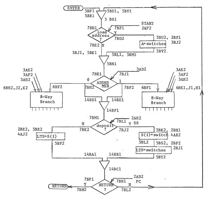
Connect 3 outputs from the 8-way branches to the address inputs of the scratchpad memory module. Only connections for  $\mathbf{S}_0$ ,  $\mathbf{S}_1$  and  $\mathbf{S}_2$  are necessary. These connections are:
