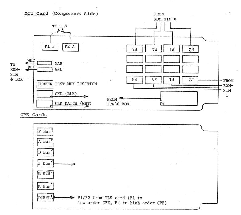
\*The I bus is connected using a three plug daisy chain cable. 16 bits are picked off from the TLS card and 8 bits are connected to each CPE card. Connect cable and make sure I bus is displayed properly as the contents of the thumbwheel switches.
