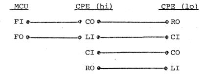
On CPE (hi) (slot 6) connect RO (HI) to LI (LOW) (pin 5BDl - 5BEl) to use the CPE card as 8 bit CPE.
